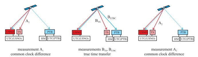
Figure 1. Schematic representation of the setup of a travelling TWSTFT station (TS) sequentially operated at USNO and PTB in three steps; the red arrows indicate the time transfer performed during the calibration with the TS. The blue line indicates the permanent TWSTFT links that are calibrated that way. Full lines indicate the measurements that are necessary for calibration.
