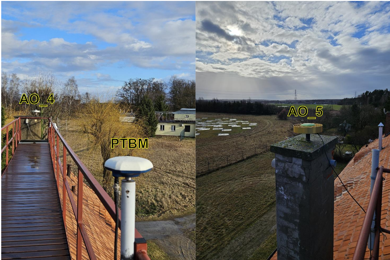
Figure 3-7 PTBM antenna installation at AOS
