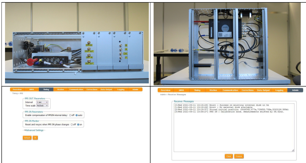
Figure 3-1 PTBM: views of the device and RxControl configuration and messages regarding PPS In and OUT.
