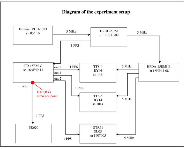
Set-up at BY was changed after the arrival of VNIIFTRI staff. Current set-up is presented on the figure above.
