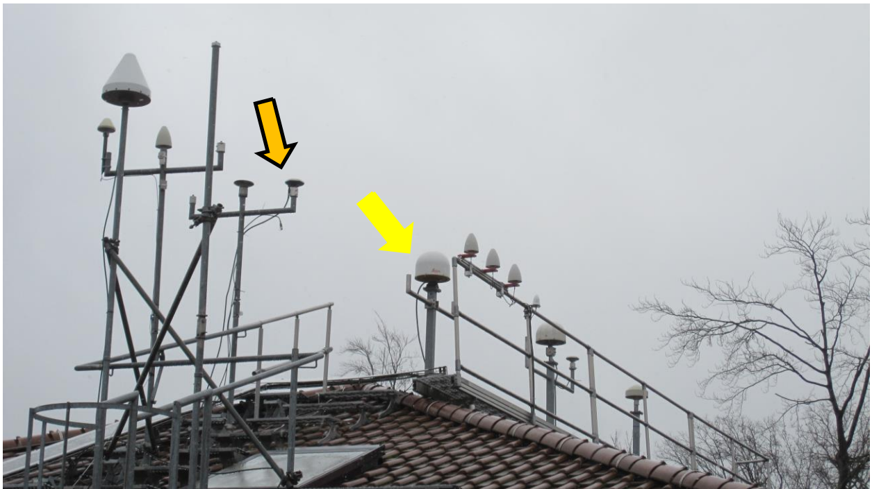
Figure 4-4 Installation of GNSS antennas at PTB, PT13 antenna (yellow) and PTBM antenna during CC1 and CC2 (orange)
