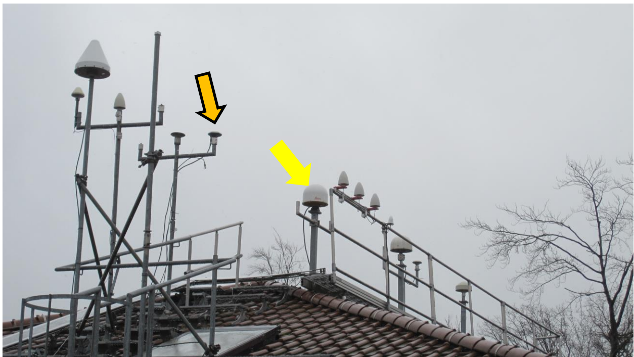
Figure 4-4: Installation of GNSS antennas at PTB, PT13 antenna (yellow) and PTBM antenna during CC1 and CC2 (orange)
