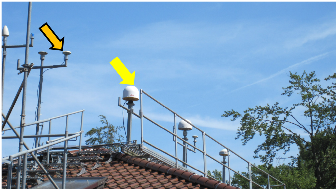
Figure 4-4: Installation of GNSS antennas at PTB, PT13 antenna (yellow) and PTBM antenna position during CC1 indicated (orange)
