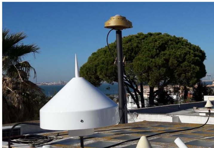
Figure 3-1: Choke Ring B3/E6 antenna on the roof of ROA laboratory.
