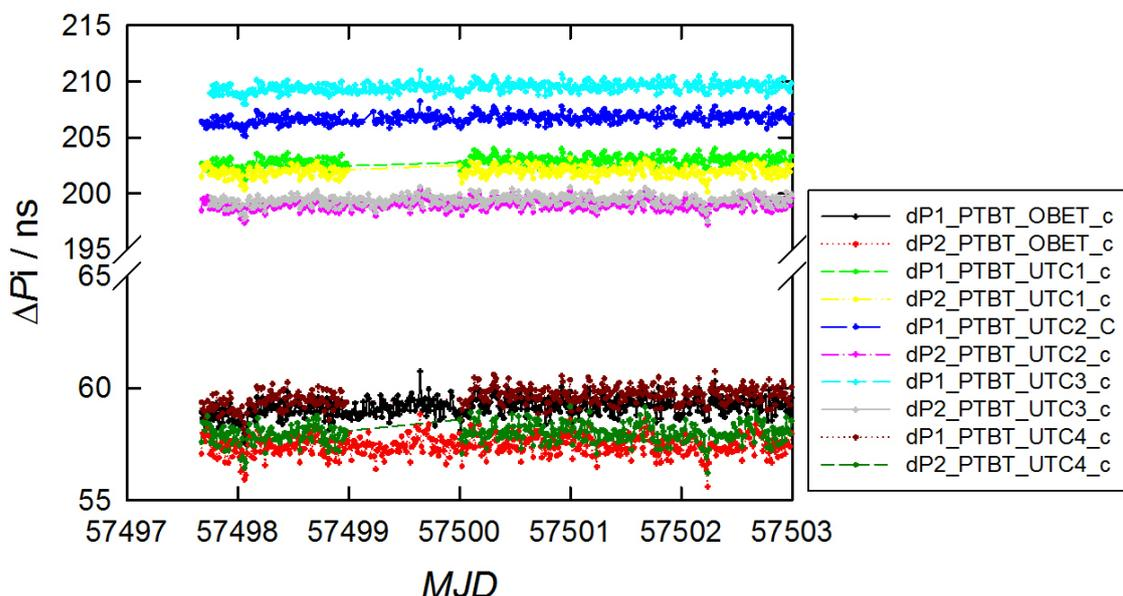
Figure 6-4:  $\Delta P_i$ -values recorded between PTBT and 5 GNSS receivers at DLR IKN, outliers and corrupted data removed
