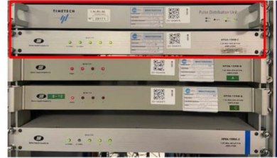
UTC(IT) TF signals to IT16, IT20 and B3TS (TimeTech Pulse Distribution Unit and SDI HPDA-15RM-C)
