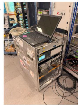
UTC(IT) TF signals to IT16, IT20 and B3TS (TimeTech Pulse Distribution Unit and SDI HPDA-15RM-C)
