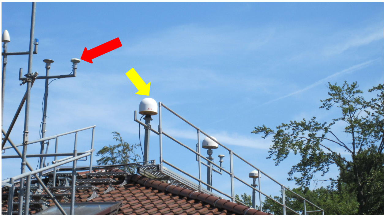
Figure 1-3: Installation of GNSS antennas at PTB, the PTBB/PT13 antenna marked yellow, the PT14 antenna red
