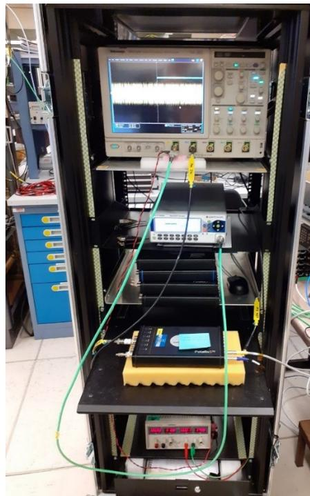
**Figure 6: Picture of the GNSS receiver calibration**
