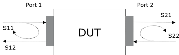
Figure 4-14 Graphical representation of S-parameters (S out - in ; out – port which analyse the output from the DUT, in – port which transmit signal into the DUT).
