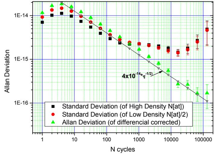
Figure 3: Allan deviation of measurements of the shift frequency in high and low atom density and their differences during MJD 53309,5 to MJD 53324,83333
