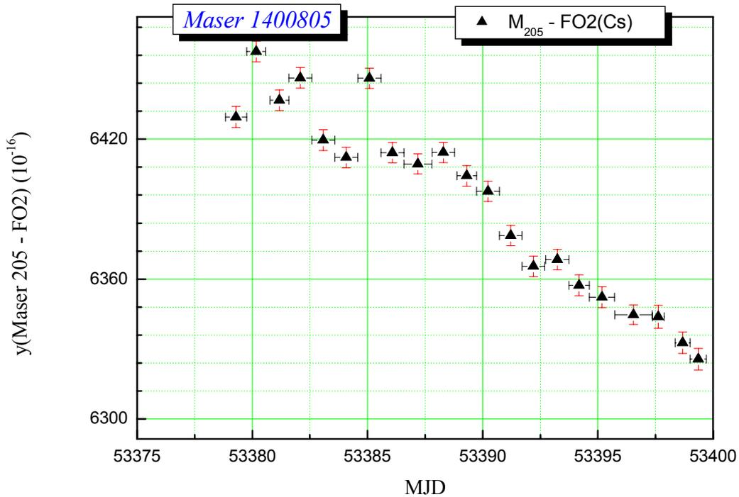
Figure 1: fractional frequency differences between H\_Maser1400816 & FO2 from MJD 53379 to MJD 53399
