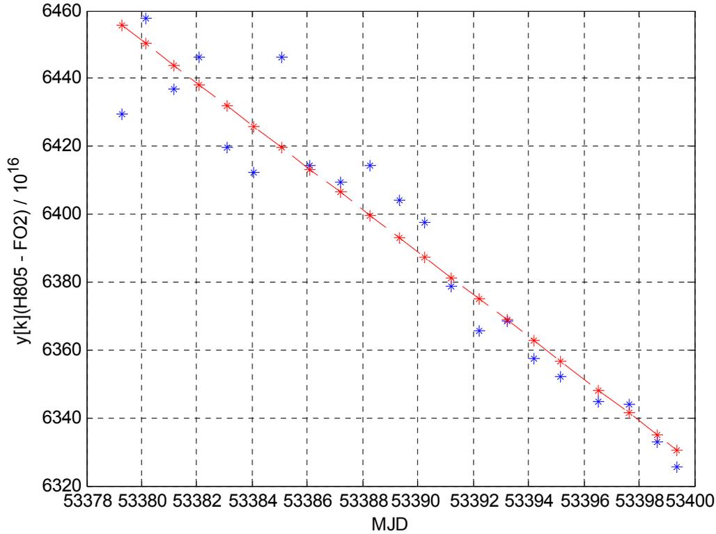
Figure 9: linear regression on the frequency  $y(\text{HMaser-FO2})$  between MJD 53379 and 53399 weighted by uncertainty :  $1/\sigma_{Ai}^2$
