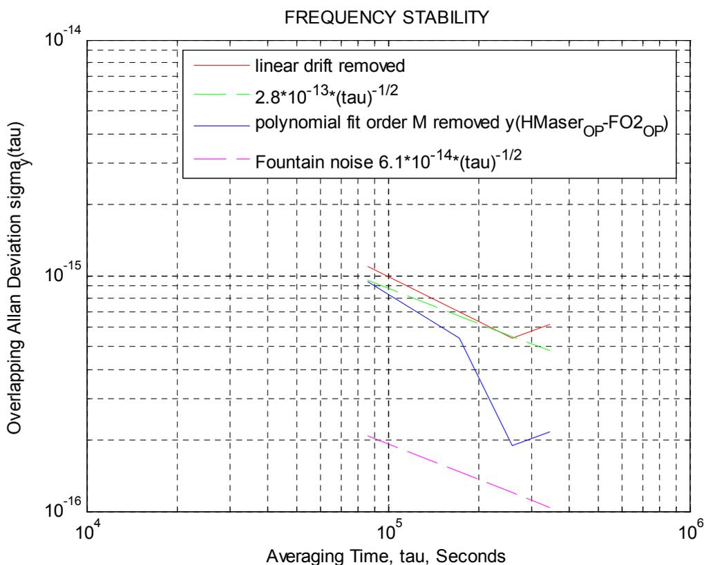
Figure 12: Comparison of frequency stability  $y(HMaser805 - FO2)$  polynomial order 2 and order  $M=11$  removed from MJD 53379 to MJD 53399
