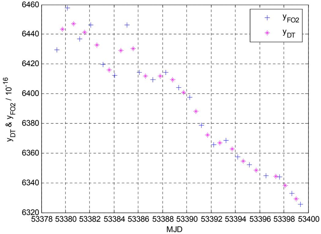
Figure 14: frequency differences H\_Maser1400805 and FO2 from MJD 53379 up to MJD 53399
