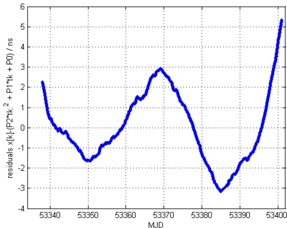
Figure 6: phase data  $x(\text{Maser805} - \text{Maser816})$  linear drift removed  $x(\text{H805} - \text{H816})$  MJD 53334 to MJD 53401
