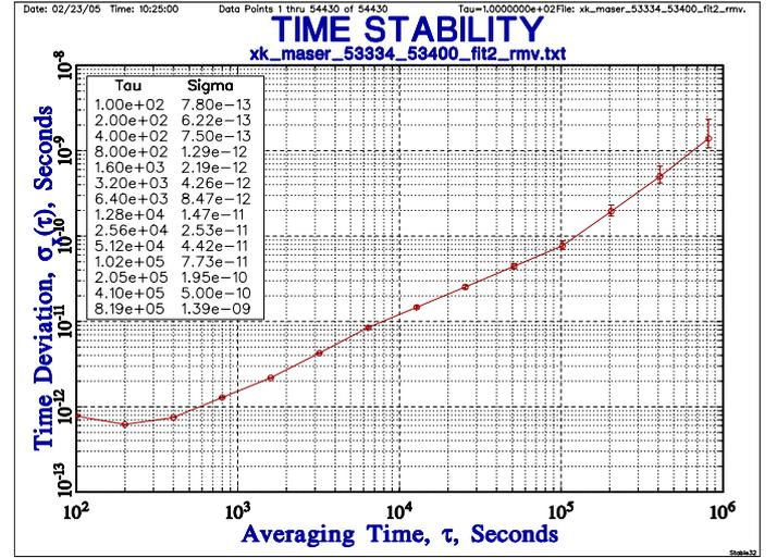
Figure 8: time stability analyzes from  $x(\text{HMaser805} - \text{HMaser816})$  from MJD 53334 to MJD 53401
