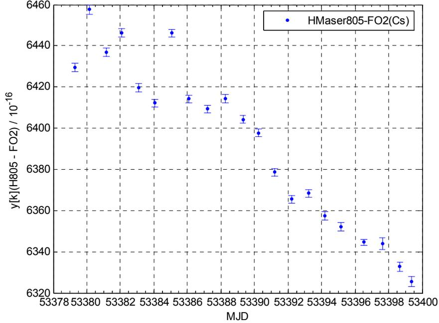
Figure 10: frequency differences averaged on about 1 day of measurements  $y(\text{H805-FO2})$  MJD 53379 - 53399
