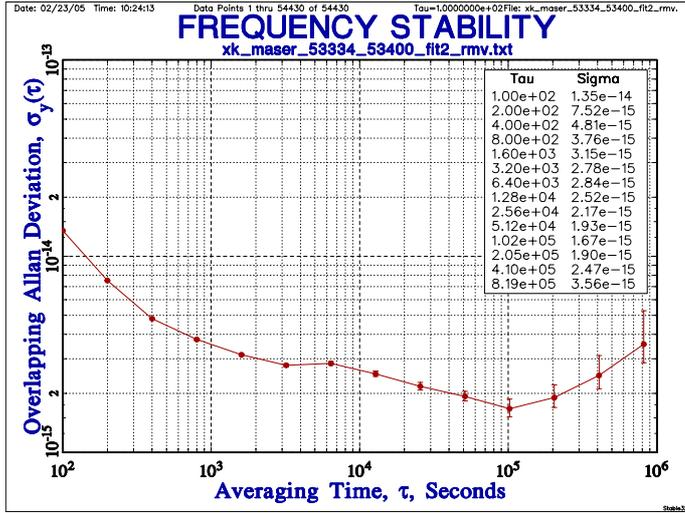
Figure 7: frequency stability analyzes  $x(\text{HMaser805} - \text{HMaser816})$  from MJD 53334 to MJD 53401
