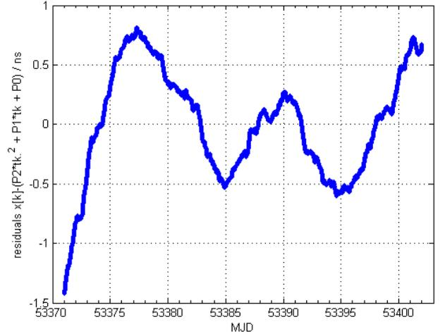
Figure 16: residuals of phase between Masers after quad fit removed, MJD 53371 up to MJD 53401
