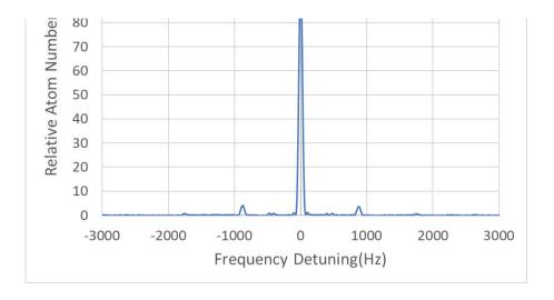
The measured asymmetry in the populations of the mF =  $\pm 1$  states is about  $2.0 \times 10^{-3}$  derived from the above figure, and the Rabi and Ramsey pulling induced frequency shift is below  $10^{-17}$  as analyzed in [3-4].
