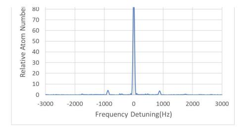
The measured asymmetry in the populations of the mF =  $\pm 1$  states is about 2.0 × 10<sup>-3</sup> derived from the above figure, and the Rabi and Ramsey pulling induced frequency shift is below 10<sup>-17</sup> as analyzed in [3-4].
