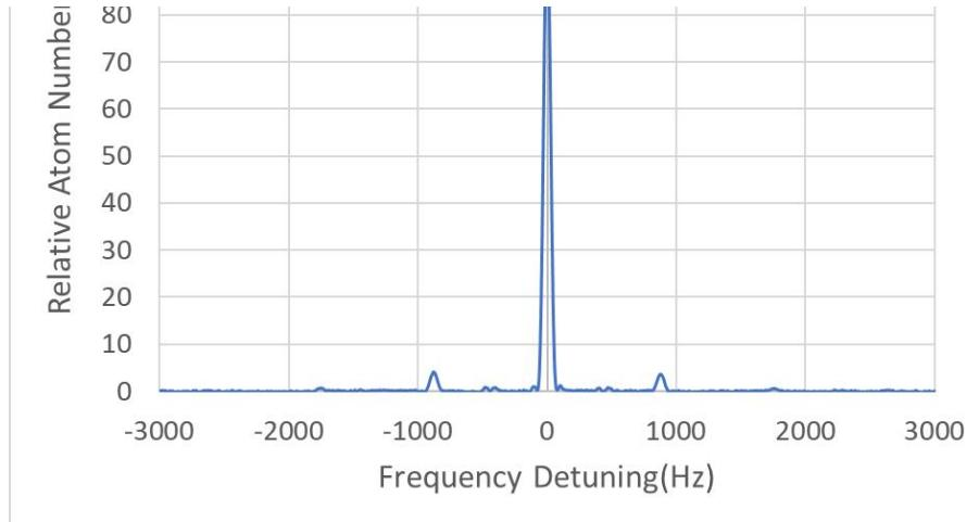
The measured asymmetry in the populations of the  $mF = \pm 1$  states is about  $2.0 \times 10^{-3}$  derived from the above figure, and the Rabi and Ramsey pulling induced frequency shift is below  $10^{-17}$  as analyzed in [3-4].
