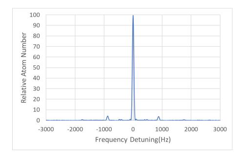
The measured asymmetry in the populations of the mF =  $\pm 1$  states is about  $2.0 \times 10^{-3}$  derived from the above figure, and the Rabi and Ramsey pulling induced frequency shift is below  $10^{-17}$  as analyzed in [1-2].
