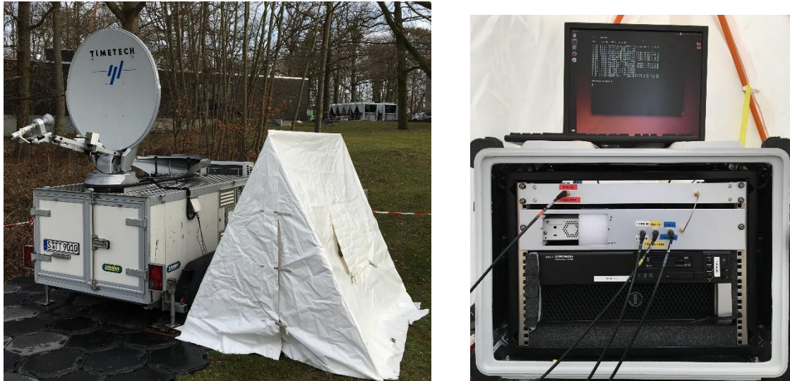
Figure 6.1 - TimeTech portable earth station and OP SDR travelling receiver installed at PTB in March 2019 during the calibration campaign
