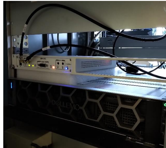
Figure 6.5 - TimeTech portable earth station installed at OP in April 2019 during the calibration campaign. The OP SDR fixed operational receiver is also shown on the right
